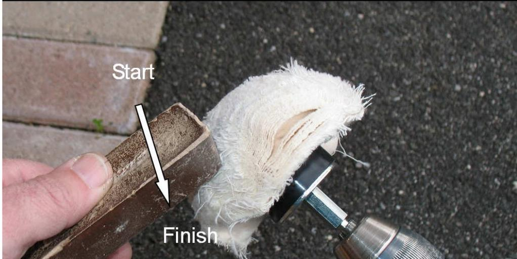
Next insert the buff into the tips and run at high speed. As you buff, apply pressure to the sides, top and bottom, moving the buff in and out at the same time. You should be spending about 1–2 minutes on each tip. Work the buff in and out with pressure. When you get towards the outside of the tip, just let the buff center in the tip, and finish the buff process. Wipe out any left over compound.
