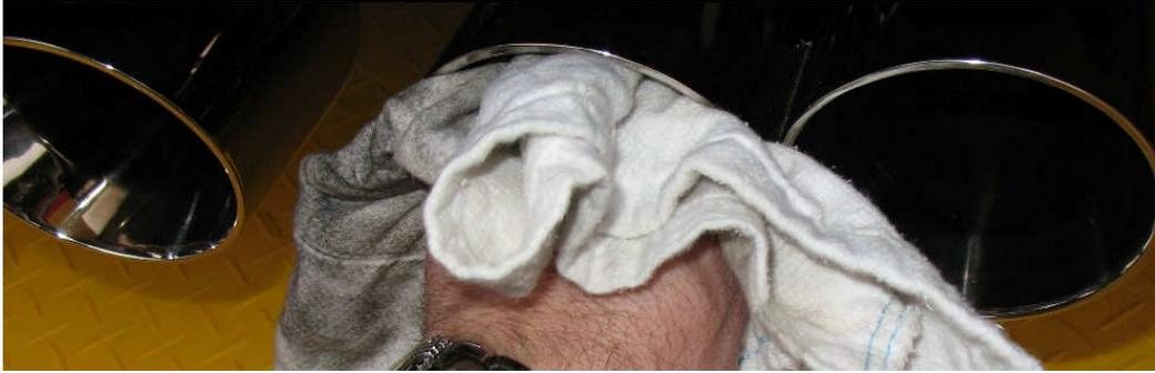
As needed if the tips get bad, repeat the *green* steps. For normal maintenance just repeat the *Simichrome* step to get back that mirror shine. Never apply wax to the exhaust pipes; it will cause them to turn yellow over time.
