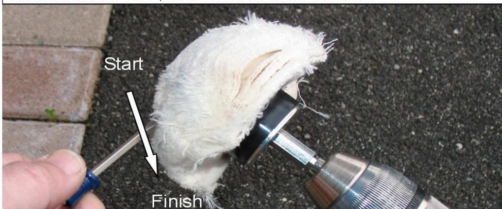
Running the drill at a high speed, apply the compound to the buff by firmly pressing the compound against the buff. It is the heat from the friction that will make the compound transfer so if it is ice cold, this could be difficult. It will not coat the buff but will leave behind the abrasive, it does not take a lot of compound.
