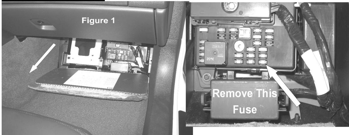
Insert the new fuse adapter into the slot you just removed the 10A fuse from. The adapter must be installed as shown with the white wire facing up and the red wire facing the center console. **Remove the grounding screw, and re-install it with the two black ground wires by inserting the screw through the connector, tighten.** Slip the control box into the location shown and place the blue antenna wire tucking it into the space shown (see fig. 2)
