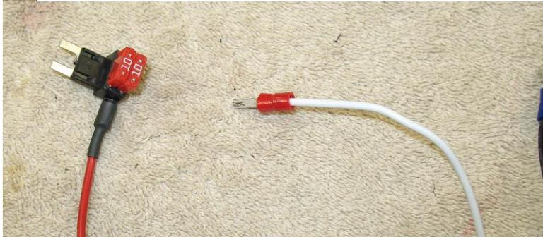
Install the 10A fuse you removed from the seat heater slot in the fuse block Yours should look like this 2 10A fuses installed in the black fuse tap and the white wire with the spade attached.
