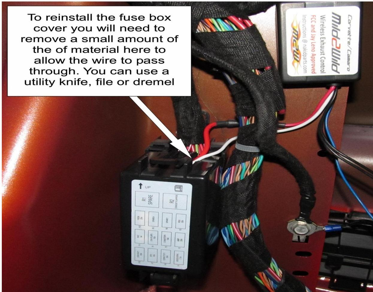
To reinstall the fuse box cover you will need to remove a small amount of the of material here to allow the wire to pass through. You can use a utility knife, file or dremel
